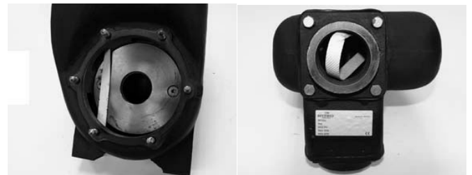
Place spacer between wear plate and impeller and do not remove until bolted to drive shaft
